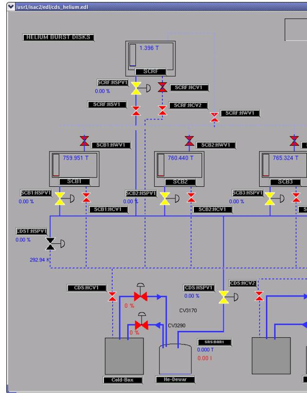
Figure 2: EPICS EDM Synaptic Display of Cold Distribution System (2 cryomodules cropped for clarity)
